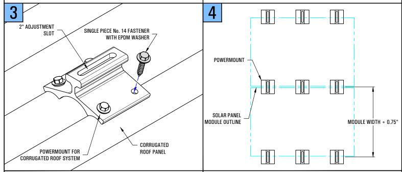
SECURE THE POWERMOUNT TO THE ROOF PANEL BY SCREWING THE SELF-TAPPING STAINLESS STEEL FASTENERS INTO/THROUGH THE PRE-PUNCHED HOLES, INTO THROUGH THE EPDM GASKET, AND INTO/THROUGH THE ROOF PANEL. MAKE SURE TO NOT OVER-TIGHTEN AS YOU WILL RISK STRIPPING THE FASTENER. IF A FASTENER IS STRIPPED, REMOVE AND REPLACE WITH A SIMILAR FASTENER, BUT OF A LARGER DIAMETER TO ENSURE PROPER INSTALLATION.
